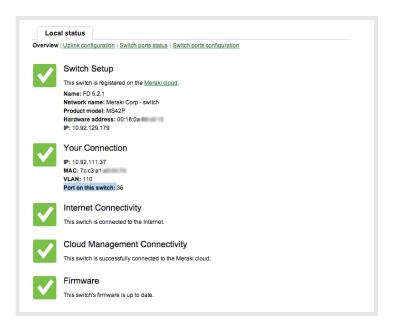
This local switch page shows the tested wall jack terminates on port 36 of switch FD 5.2.1.
