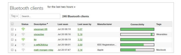
The current online status, description, manufacturer, and connectivity statistics of Bluetooth devices are displayed within the Meraki dashboard for APs with BLE enabled.
