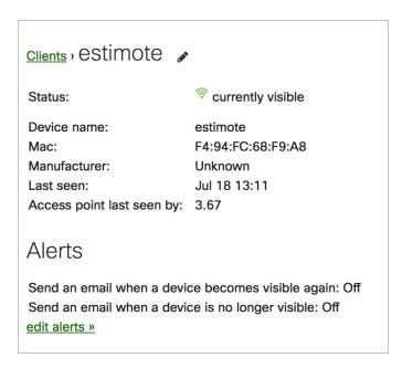
It's possible to configure email alerting within the Meraki dashboard for BLE-capable devices.
